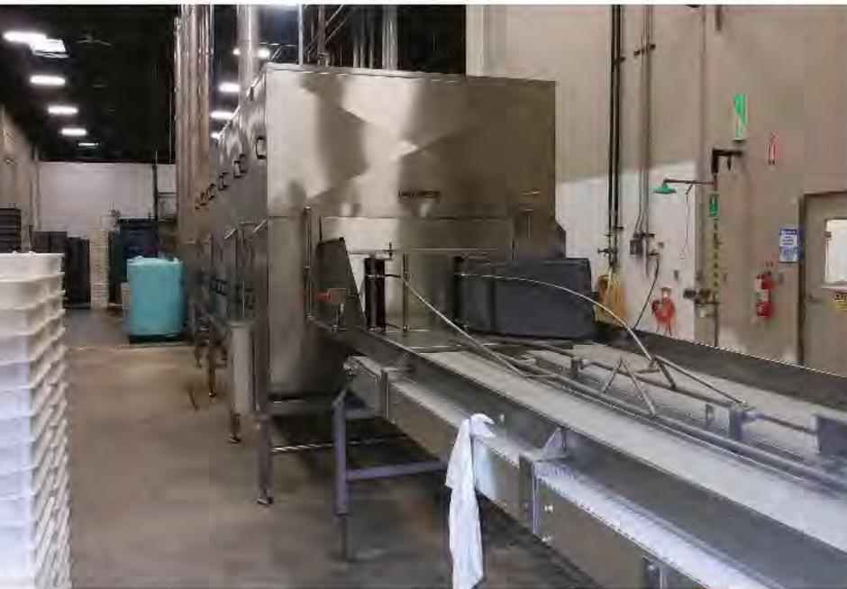
Papa John's Dallas commissary installed an automated two-lane, four-tank washing system provided by CM Process Solutions to clean and sanitize 2,000 dough trays an hour.
